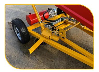
**Option:** : valve block control on both sides of the belt
