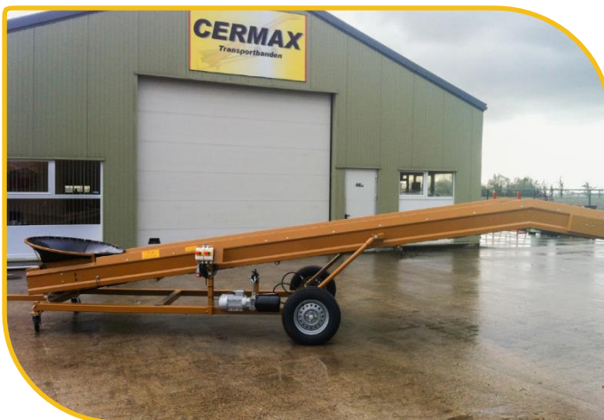
Option: hydraulic power unit with valve block, sprayed in a different colour
