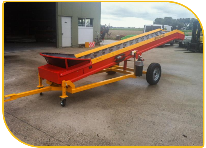
Option: mechanical infeed height adjustment
